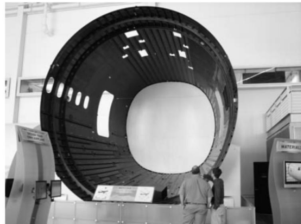
A cured 787 fuselage barrel section
