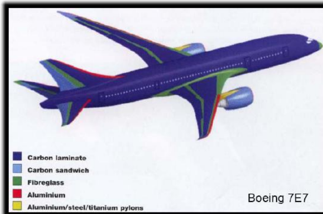
Composite use in the Boeing 787
