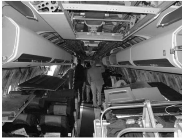
Figure 2-49: The Cabin of a Boeing 757 During Parting-Out
